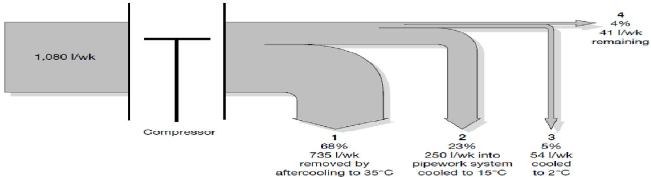
**Fig 4. Ref – Good Practice Guide 216 – Energy saving in Drying of compressed Air – 68 % water removal in Air cooler**
