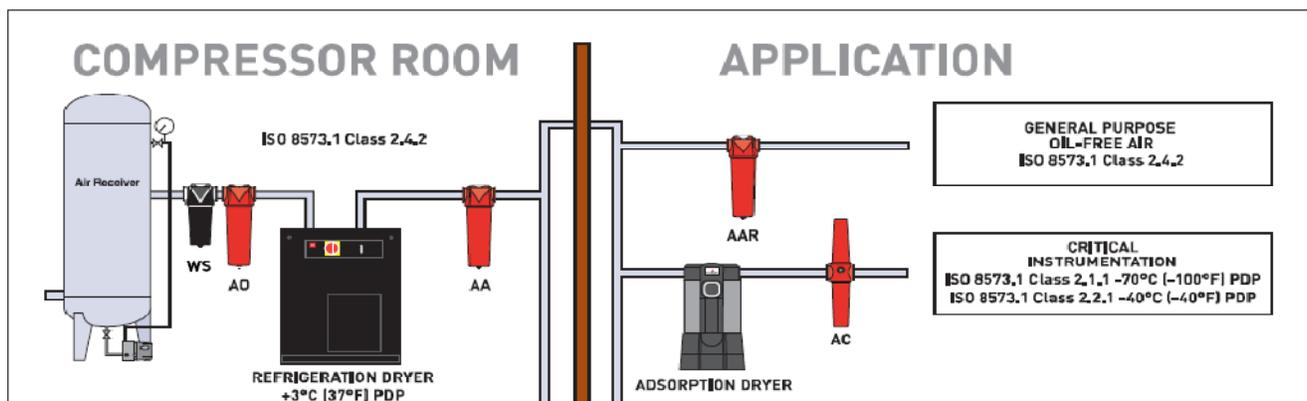
Fig.3.– Location of WS after the wet receiver & before Dryer - Reference Parkar compressed air treatment manual.
