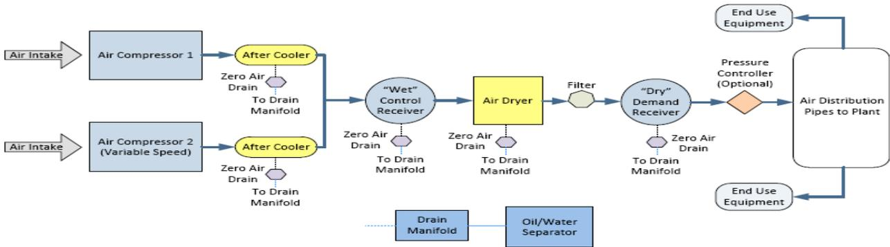
**Fig 1 – Compressor & compressed air treatment sub systems to stand alone with buffer as two air receivers.**
