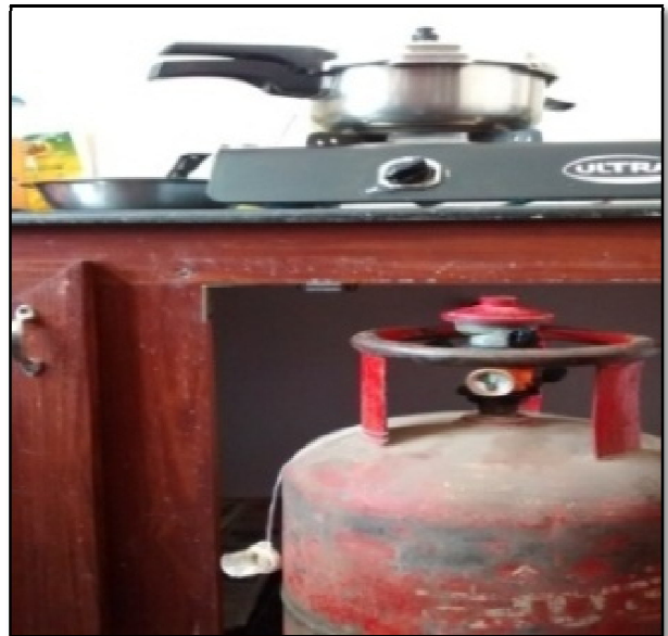
DEVICE FITTED ON CYLINDER TOP BEFORE EXISTING REGULATOR
