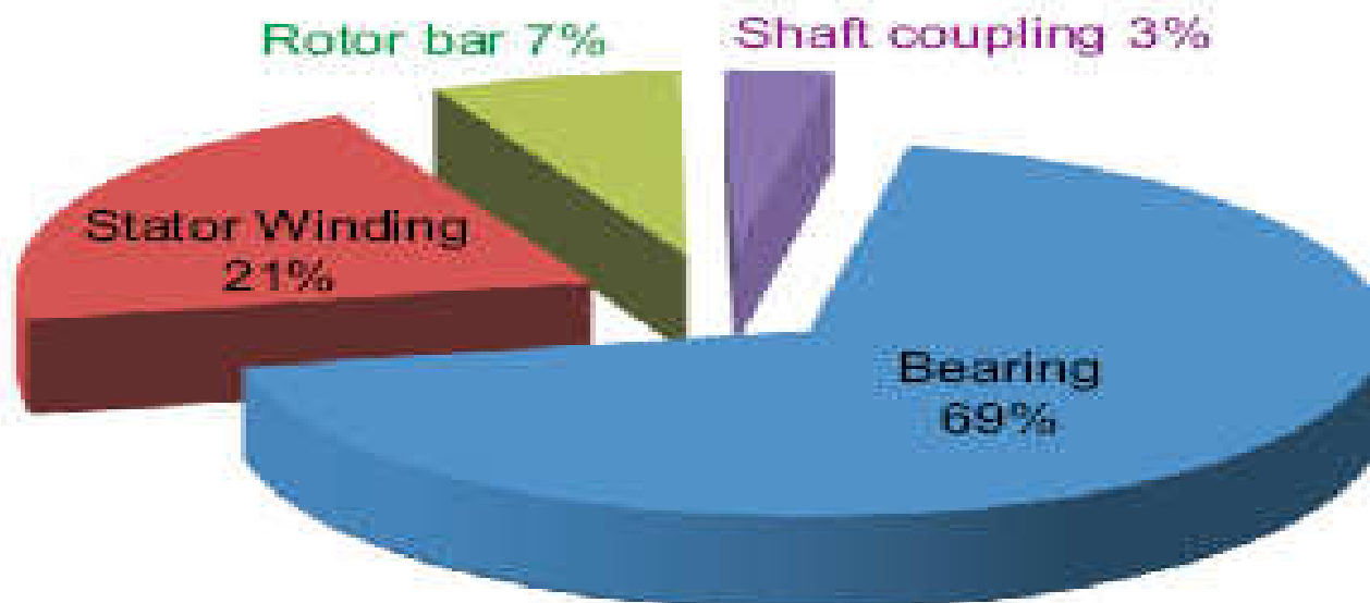
Fig. 5. Extrapolated distribution of failure by motor component
