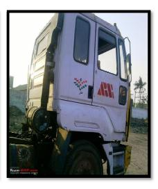
Image I – Autorickshaw, where the Pre-filter is elevated at the rear by piping to top, from Air Intake filter near Engine. Image II – Washable Pre-filter provided on top of Tractor Engine, the same to be fixed to Autos & other 4 wheelers. Image III- in HCV, the Pre-filter is elevated at 3 meter Height by piping from the existing air filter near the Engine.
