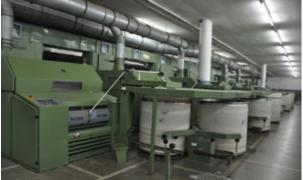
Though the WRS OEM has given the Pascal gauge at the filter box, and at the individual cards, the mill has to maintain the optimum Pascal suction at each of the card. Since the same is not condition monitored routinely, the mill is losing heavily in the WRS and now each mill is finding this proposal as a Low Hanging Fruit in ECON measure.
