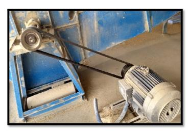
VII image Cogged belting done in this machine, see the right size of belts, pulley sizes and the Angle of Arc contact. VIII image See the Motor & Load Pulley sizing – cogged belts rightly matched to look in STILL motion in Run mode.
