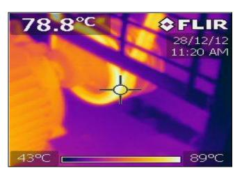
III image shows excess weight in pulley and more number of belts in 30 HP rated Rice Polisher machine. IV image shows the thermal imaging of worn-out pulley due to belt and alignment issues raises temperature to 89 \*C. This Thermal Image of belt & pulley will show how much your KW input to motor is unwantedly heating up the belts & pulley drives. You will also find rubber burnt smell and screeching sound when machine is started and these are the signs of wear-out happening.
