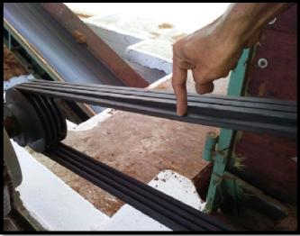
V image – Cogged Belts and Drives rightly changed for this motor drive system and Energy savings achieved. VI image Belt Tension must be in such a way that when pressed, it must not exceed the belt thickness here.
