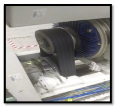
I image shows short ring frame runs with loose belts on the pulley and not gripping, hence losing the RPM in belt transmission. II image shows in the Long ring frame, the heated belt, pulley and hotter motor Drive-end bearings, all Hot Spots show Loss. III image – OEM's Latest machines have Timing belt along with reduced pulley sizes for power saving and no RPM loss now.
